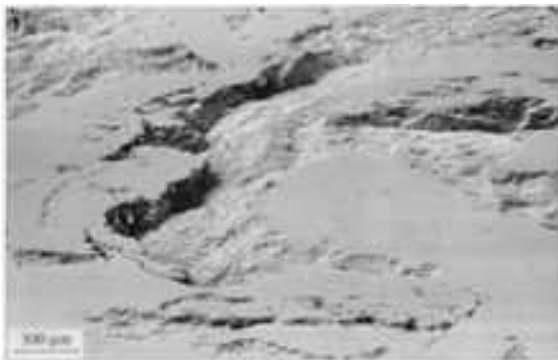
Fig. 19 Scanning electron micrograph revealing two damage mechanisms on a steel cam follower, run against a steel cam. Smoothing by plastic deformation and wear by surface fatigue-induced fracture. Note the surface cracks partially surrounding the wear craters.
