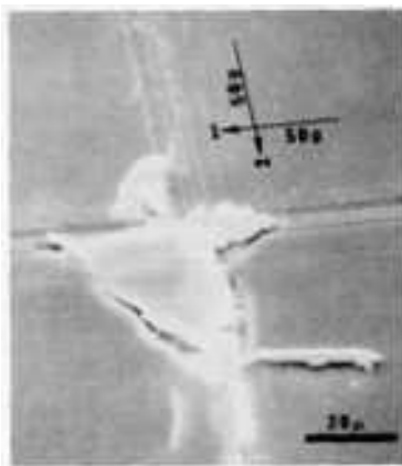
Fig. 7 Intersecting wear tracks on a fluorapatite single crystal under a 0.5 N load. Source: Ref 43
