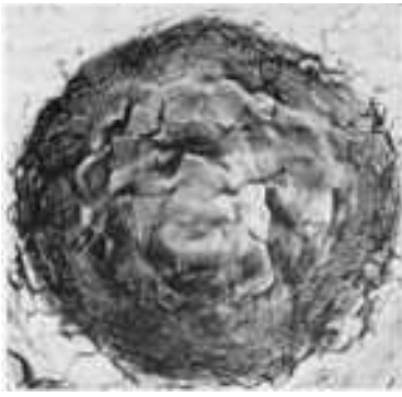
Fig. 6 Deformation due to a single impact on aluminum impacted by a short discrete jet of water at 750 m/s (2460 ft/s). Note the central depression, which is of similar diameter to the impacting jet, and the circumferential surface ripples surrounding it. Courtesy of J.E. Field, Cavendish Laboratory, University of Cambridge, United Kingdom
