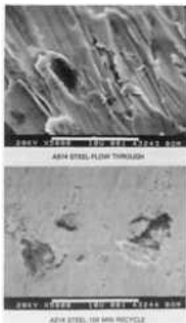
Fig. 5 Comparison of wear surfaces for low-alloy steel specimens worn in flow-through (top) and recycled (bottom) slurry tests for 1 h and 1.67 h, respectively. Source: Ref 13
