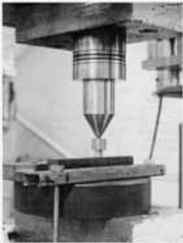
Fig. 12 Button-on-block galling test. Source: Ref 23
