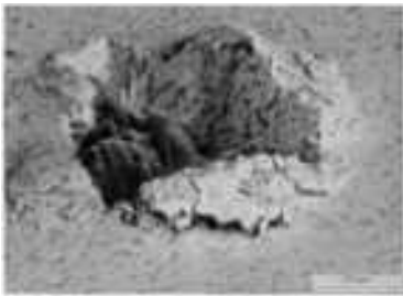
Fig. 6 Scanning electron micrograph showing plastic deformation without material loss in a cemented carbide surface exposed to single-particle impact. The binder phase (cobalt) has been extensively plastically deformed, while the hard carbides have been pushed around without deforming but have occasionally partially deadhered from the matrix. The surface has also been damaged by the pickup of fragments from the erosive SiC particle. Courtesy of Mikael Olsson
