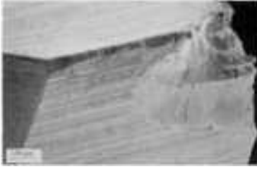
Fig. 15 Scanning electron micrograph showing brittle fracture of a cemented carbide tool tip used to cut aluminum
