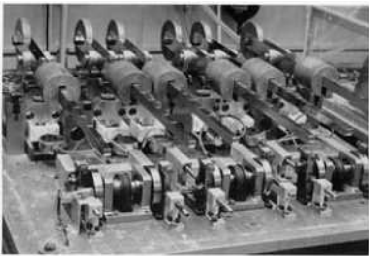
Fig. 6 Six-station reciprocating pin-on-plate friction and wear machine used to evaluate prosthetic implant materials
