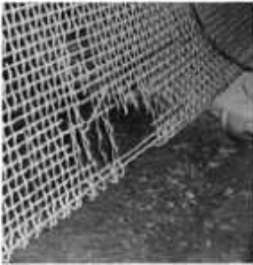
Fig. 1 Worn wire screen in minerals processing plant showing effects of sliding wear in moist environment
