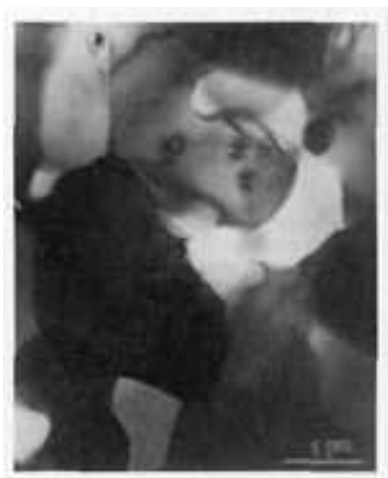
Fig. 18 Bright-field image of a polycrystalline aluminum alloy
