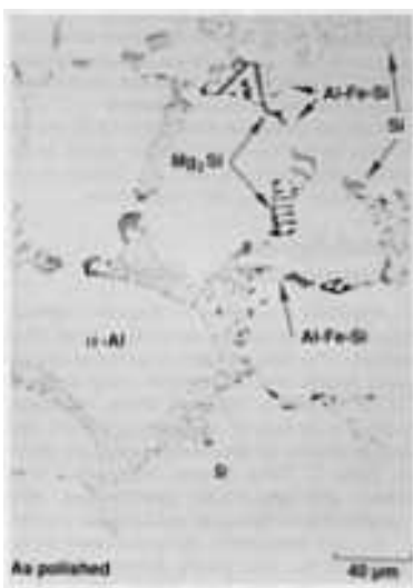
Fig. 2 Typical microstructure of type A357.0 hypoeutectic alloy. Source: Ref 11
