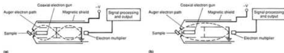
Fig. 14 Cylindrical mirror analyzer types. (a) Double pass. (b) Single pass
