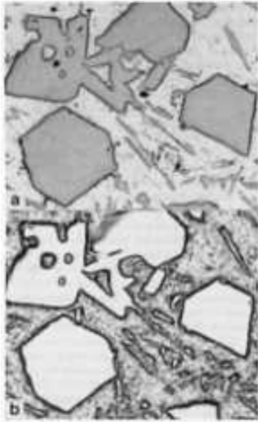
Fig. 7 Optical micrographs of an Al-13Si alloy polished in a dry abrasive and an abrasive entrained in a water slurry. (a) Diamond abrasive applied so that the grits were held fixed to the fibers of a polishing cloth as shown in Fig. 6(b). Alumina abrasive of a grade corresponding to diamond but applied as a water slurry. The fixed diamond grits operated in a cutting mode and cut extended grooves in both the hard silicon phase (angular light gray) and the soft aluminum phase of the matrix. The loose alumina grits, presumably operated in an erosive mode, produced only indentations in the aluminum phase, which consequently has a comparatively poor reflecting matte finish. Both 500×
