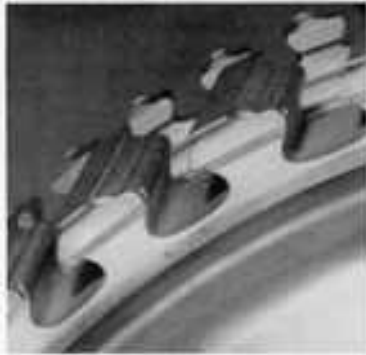
Fig. 6 Front-stage HPC rotor disk showing dovetail disk slots and pressure faces
