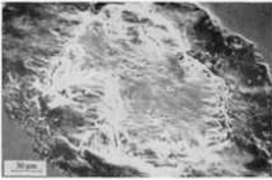
Fig. 20 Scanning electron micrograph showing surface damage in stainless steel, typical of fretting-induced fatigue fracture. A crack loop surrounds the unaffected stick patch.
