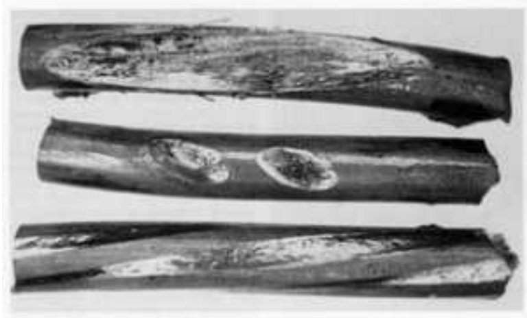
Fig. 3 Wear scars in steel wire segments cut from inner strands of a severely internally worn wire rope used in dragline operations. (Top) Long scar typical of low-angle cross-wire contact. (Middle) Scar typical of high-angle cross-wire contact. (Bottom) Longitudinal scar caused by plastic deformation of contacted wires within the weave
