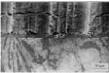
Fig. 25 Scanning electron micrograph showing the top surface and cross section of a hot roll with a protective oxide layer transferred from the heat (work material). As long as the layer adheres to the roll surface, the oxide coating protects the underlying metal efficiently by continuous pickup of oxide at the same rate as the simultaneous loss by wear. Courtesy of Lynn Erickson
