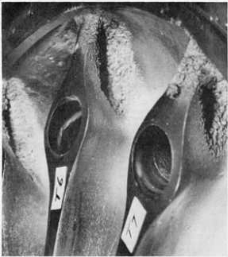
Fig. 3 Severe erosion of copper-manganese-aluminum stator vanes in a hydraulic dynamometer. Each vane has lost about 10 cm 3 (0.6 in. 3 ) of material. See text for a discussion of the erosion mechanism.
