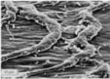
Fig. 14 Scanning electron micrograph showing roll formation associated with tearing of material from the surface of polyurethane during sliding against a flat metal surface. Sliding direction of counterface was from left to right.
