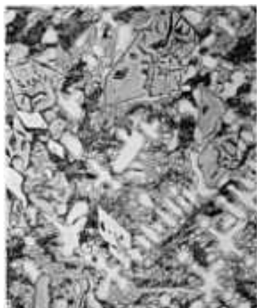
Fig. 11 Microstructure of ERNiCr-C (two-layer PTA deposit) nickel-base/boride-type nonferrous alloy. 425×
