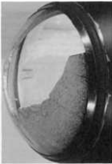
Fig. 2 Rain erosion effects on a Maverick missile dome made of coated zinc sulfide that was exposed for 10 s at a speed of about 210 m/s (690 ft/s). The dome itself suffered catastrophic damage, and erosion is also seen on the filled elastomeric mounting ring. Courtesy of G.F. Schmitt, Jr., Materials Laboratory, Wright Research and Development Center, Department of the Air Force
