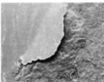
Fig. 34 Typical delamination in the fretted region produced by metal-to-metal contact
