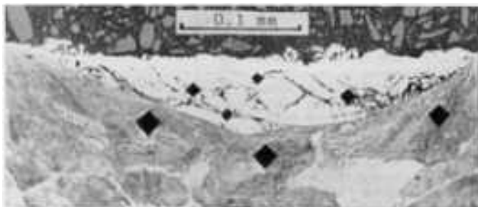
Fig. 21 Cross-sectional view of a white layer of martensite produced by fretting of a carbon steel connecting rod. Axial stress, 0 to 380 MPa (0 to 55 ksi); contact stress, 40 MPa (6 ksi); fretting cycles, 10 5 . Sample was
