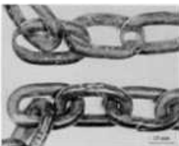
Fig. 21 Wear by corrosion and shear fracture of two sections of a galvanized steel chain partly submerged in water. Note the extreme difference in wear rate between the underwater (top) and above-water (bottom) links, caused by the synergistic effects between corrosion and wear. The general corrosion rate was low.
