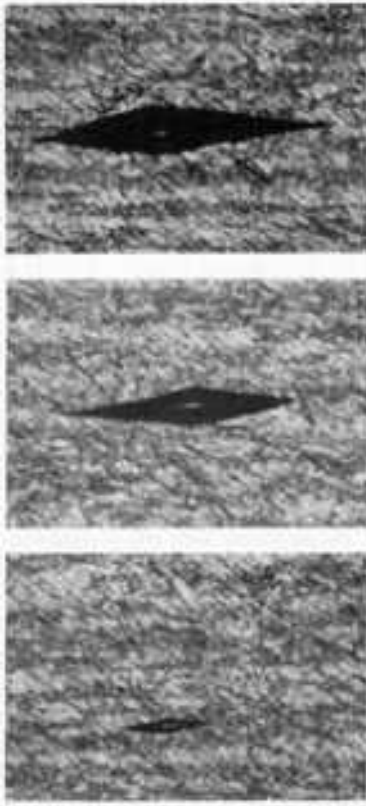
Fig. 8 Diamond-shaped (Knoop tip) indents before and after polishing. Longest indent is about 31 \mu\text{m} (1.2 mils) long and 1 \mu\text{m} (40 \mu\text{in.} ) deep.
