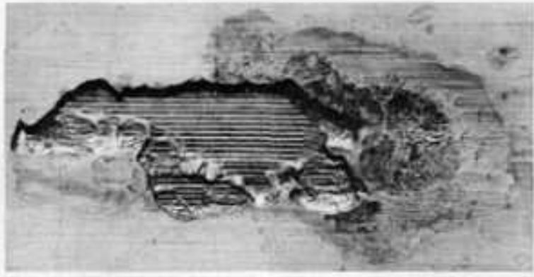
Fig. 1 Macrograph of a spall in a babbitt metal journal bearing. 8×
