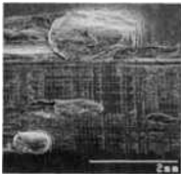
Galling on the surface of type 316 stainless steel rubbed against a button of the same material at a load of \sim 1000 N. Courtesy of L.K. Ives, NIST
