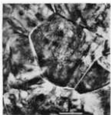
Fig. 22 Accumulation of dislocations near grain boundaries caused by sliding contact. The material is \text{Al}_2\text{O}_3 doped with MgO. Source: Ref 53
