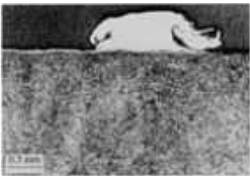
Fig. 23 Optical micrograph of cross section of a patch of wear debris on a quenched and tempered steel surface, transferred from the high-speed steel (HSS) counterface during sliding contact in a crossed-cylinders test. Having been in constant contact with the countersurface and thus frictionally heated to a higher temperature, the normally more wear-resistant HSS material has been worn by adhesive shear fracture, while the countersurface has been damaged by the transferred debris. Courtesy of Mikael Olsson.
