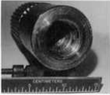
Fig. 3 Valve stem nut showing wear of threads
