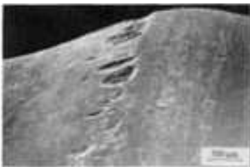
Fig. 3 Scanning electron micrograph of a thread of a percussion drill coupling. Mild abrasive and coarse pitting wear mechanisms dominate the wear to a fraction of 85% and 15%, respectively.
