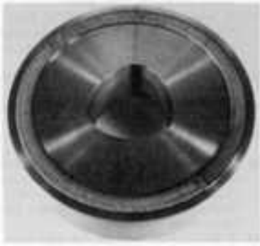
Fig. 22 Inconel alloy shaft seal test ring particle-injected with WC. Source: Ref 63
