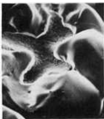
Fig. 12 Scanning electron micrograph of a composite restoration (Concise) with severe occlusal wear after a seven-year period. 10 \times . Source: Ref 188
