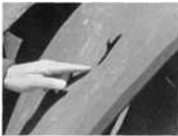
Fig. 3 Worn cone crusher liner after 3 months of use
