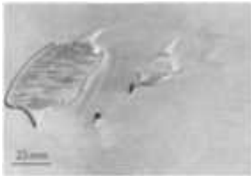
Fig. 6 Surface tears caused by fretting damage when aluminum cylinders in Fig. 5 are extruded
